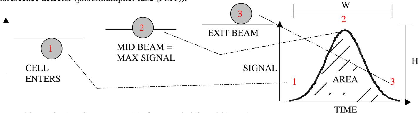
The resulting pulse has three measurable features: height, width, and area.
