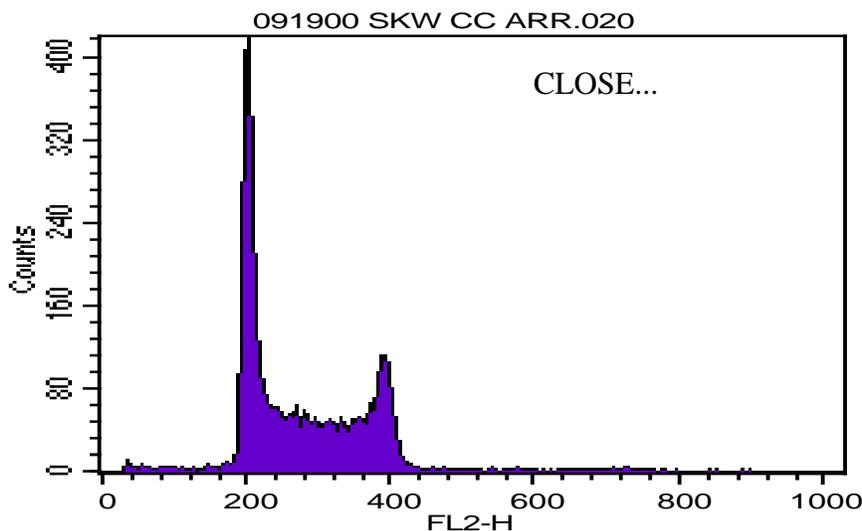
This is a histogram of FL2-Area (total cell fluorescence). This graph looks VERY similar to the FL2-H histogram. Although it is showing us the correct parameter for DNA analysis, it still does not allow for aggregate discrimination.
