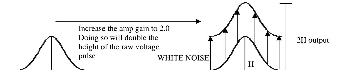
The amp gain on a flow cytometer ranges from 1.00 (no alteration of raw voltage pulse) to 9.99 (nearly 10 times the amplification). On FSC, if you need to amplify more than 9.99, you adjust the rough voltage setting to the next step (a ten-fold increase) and bring your FSC Amp gain setting back down to 1.00 – and then adjust your amp gain as necessary.
