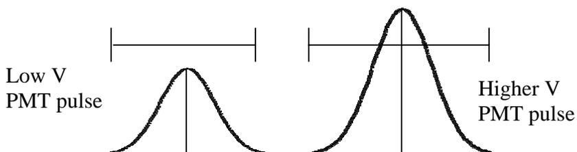
By increasing the PMT voltage, you can change a pulse's height, width and area values
